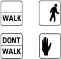
A pedestrian signal allows a safer way for pedestrians to cross the street at signalized intersections. The pedestrian signal, when activated, provides time for the pedestrian to enter the street on the steady “Walk” and to finish crossing the street on the flashing “Don’t Walk” signal. The pedestrian signal is normally activated by a pedestrian detector push-button, that causes the controller to operate a pre-programmed timed sequence of steady “WALK” and flashing “Don’t Walk” signals.
