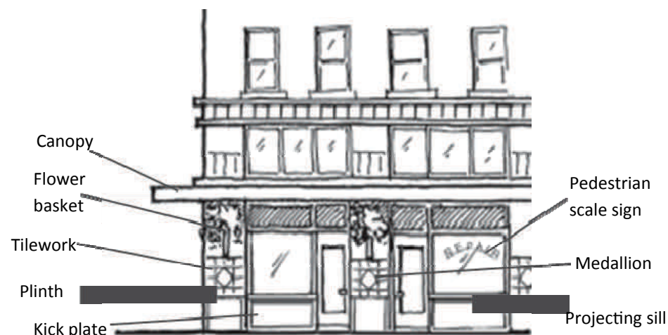
Elements used at ground level
