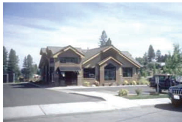
6 inch vertical curb defines pedestrian connection
