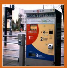
OFF-BOARD FARE KIOSKS Off-board fare collection enables all-door boarding, speeds up the boarding and alighting process and saves valuable time for all passengers
