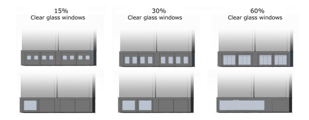
**Figure 6.4.1 -** Especially along pedestrian-oriented streets, glazing provides a visual connection between activities inside and outside a building. Table 6.4.1 specifies minimum quantities of clear glass, expressed as a percentage of each façade.
