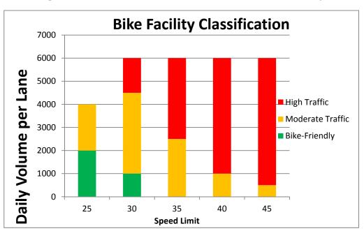
Figure 2. Bike Route Classification based on traffic volume and speed
