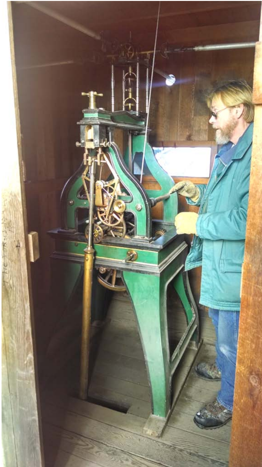
Photo of the Clockwork Mechanism that Shows Connections to the Pendulum Below, the (4) Clock Face Drive Shafts at Top, and the Counterweight Cable Running up to the Mid-Right
