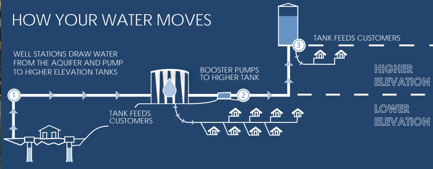
**1** The City of Spokane has seven wells located throughout the City from which it draws water directly from the aquifer. The water from the aquifer is pure enough to be pumped directly from the ground without any treatment. We simply add chlorine to the water to ensure that purity is maintained throughout the distribution system.
