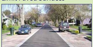
Narrowing street widths, using pervious pavement, and reducing building footprints may result in smaller storm drainage facilities.
