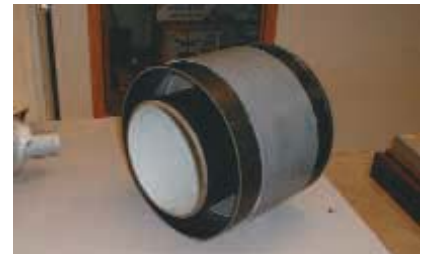
Figure 20 Large, steel, double-wall piping.
