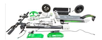
Lime's vehicles are designed to be modular, with every piece able to be removed and replaced. Only when vehicles experience damage such as extensive vandalism which compromises the frame are they considered beyond repair. In those cases, our Operations Team disassembles the vehicle to separate aluminum, plastic and electronic component parts for repair and reuse on other vehicles. Parts unsuitable for repair are then recycled.
