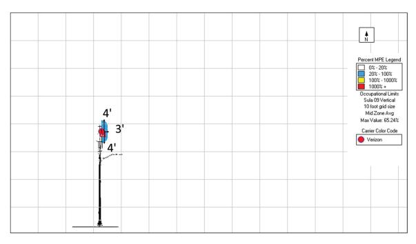
The **General Public** safe clearance zone for a standard Verizon antenna located within 3' in front (Horizontal) of Verizon antennas. This safe clearance zone also includes anywhere within 4' above and 4' below (Vertical) each Verizon antenna's centerline when also located in front of the antenna
