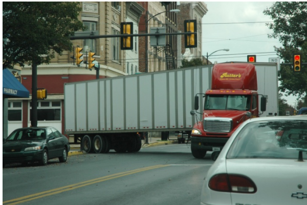
Figure 29 – Infrequent accommodated vehicle can encroach into opposing lane
