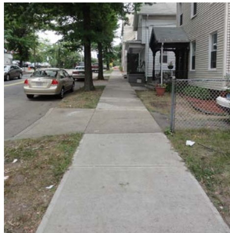
Figure 19 - Continuous Sidewalk Design Establishes Pedestrian Space over Driveway
