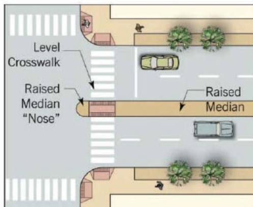
Figure 23 - Protecting crossings with a median tip provides safety from turning traffic.
