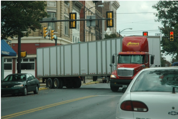
Figure 25 – Infrequent accommodated vehicle can encroach into opposing lane
