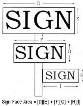
FIGURE 4 Sign Face Measurements
