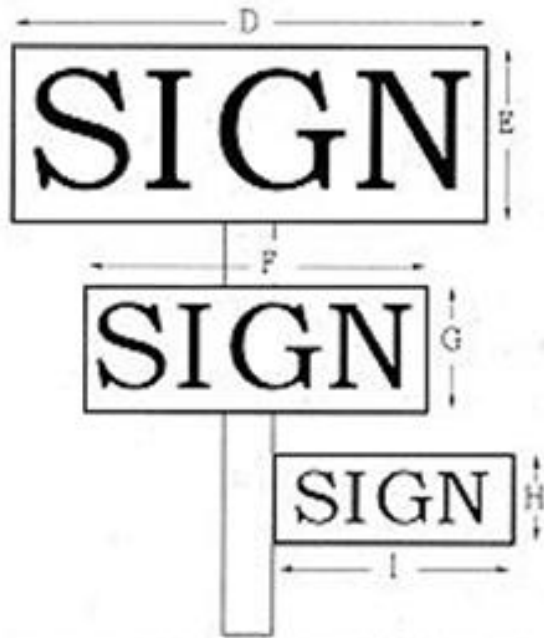
FIGURE 4 Sign Face Measurements
