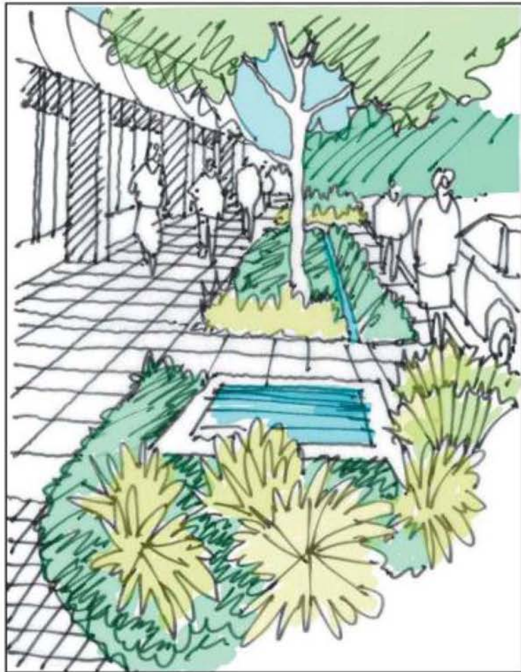
Rain gardens with native plantings integrated into an urban streetscape
