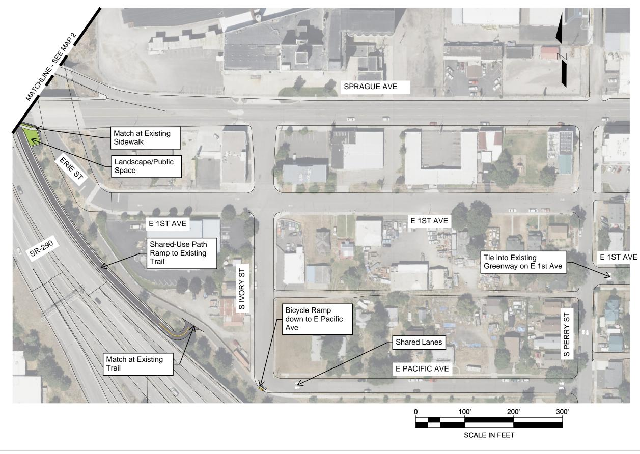
THIS IS A PRELIMINARY CONCEPT. FIELD VERIFICATION, SITE CONDITION ASSESSMENTS, ENGINEERING ANALYSIS AND DESIGN ARE NECESSARY PRIOR TO IMPLEMENTING ANY OF THE RECOMMENDATIONS CONTAINED HEREIN.
