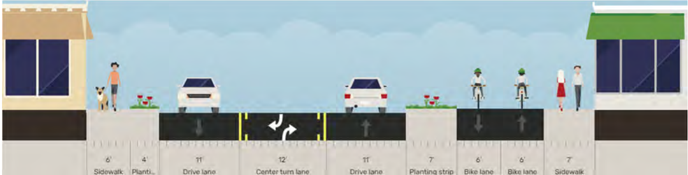
Figure 15: Sprague Avenue Proposed Cross Section (dimensions are approximate)
