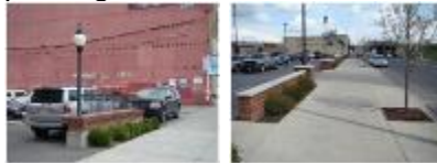
Parking liner walls with plantings contribute to an interesting pedestrian environment. The parking liner wall and screen pictured above is enhanced by larger wall sections near automobile crossing points and a change in sidewalk scoring pattern. Both give cues to pedestrians and drivers.
