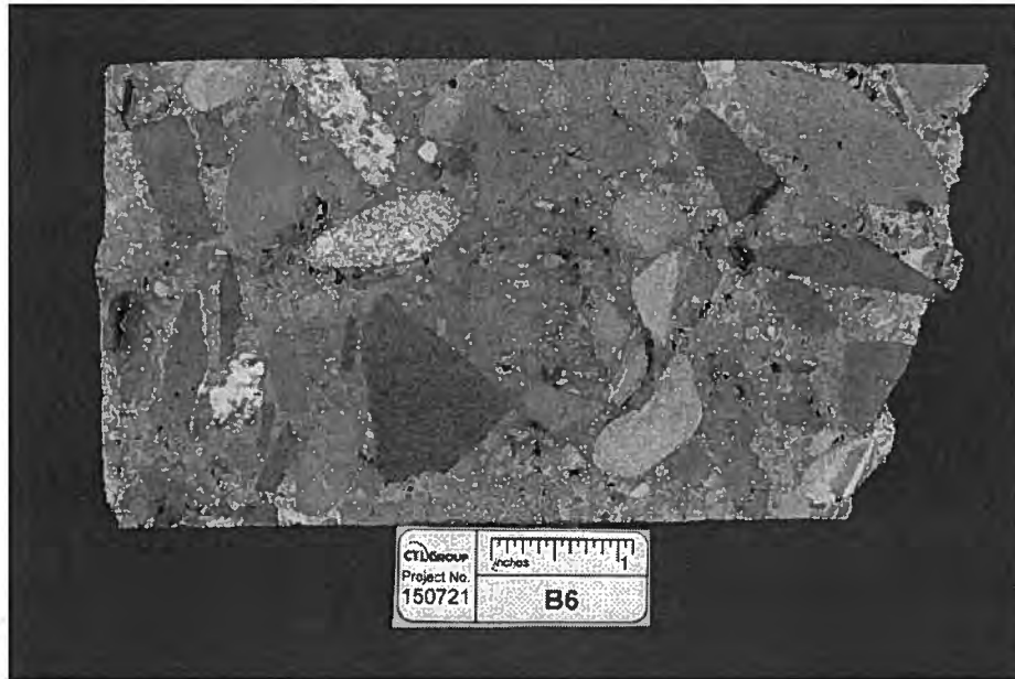
Fig. 4 Saw-cut cross-section of Core B6, exterior surface at left, stained with pH indicator (phenolphthalein) solution. The solution imparts a deep magenta stain to high pH, non-carbonated paste. Carbonated paste does not change color.
