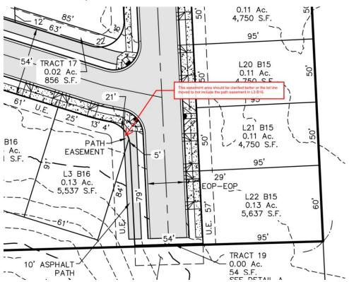
2. A sewer easement will be required for the proposed sewer connection to Lot 3 Block 16 (see snip below from construction plans).
