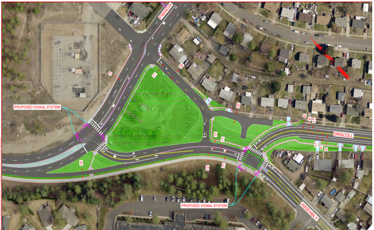
Figure 6 – Alternative D Roadway Network
