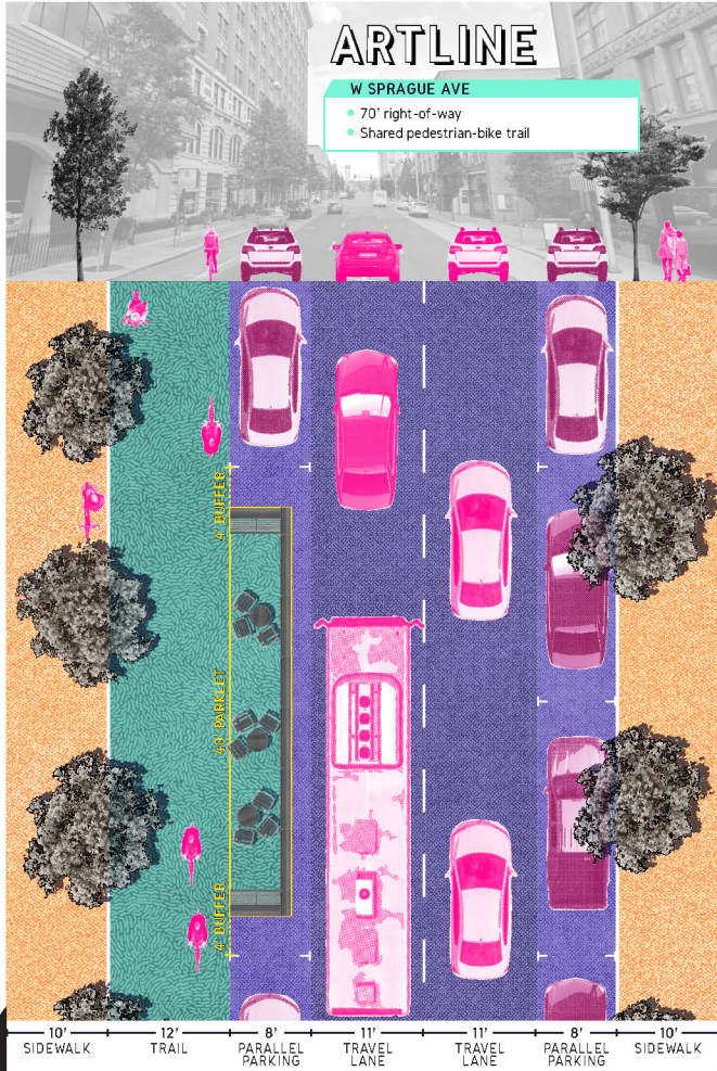
FIGURE 13 Cross-section of the long-term vision for the reconfiguration of Sprague Ave, prioritizing active transportation and public space.
