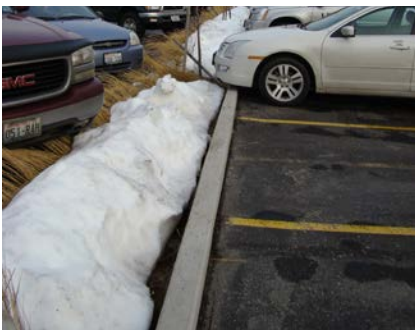
Integrate snow storage with stormwater facilities, or preferably designate parking stalls or other paved areas adjacent to stormwater facilities for snow storage.
