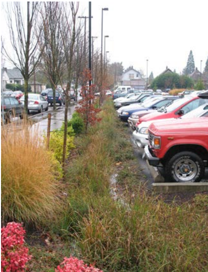
Infiltration beds can be planted with native or other plants adapted to seasonal variations in water saturation and drought.
