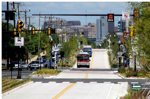
Improved traffic signal timing to efficiently move buses between stops and reduce delay at intersections.
