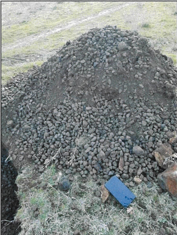
PHOTO 3: TP-1 EXCAVATED SOILS
