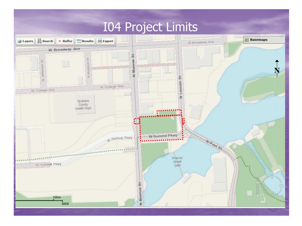
**Construct a 250'** long by 50' wide underground storage tank for excess stormwater – combined sewage
