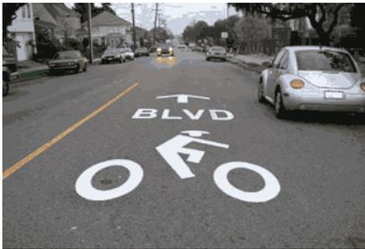
**Bike Lane:** A bike lane is identified by on-street striping. Typically a bike lane is 5 feet wide. However, bike lanes can be 4 feet wide if there is no on-street parking to the right of the bike lane. An on-street marking of a bicyclist and/or street signs identifying the bike lane may accompany
