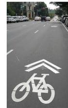
to remind all roadway users to share the road while directing cyclists out of the "door zone." On roads with steep terrain, a "climbing lane" should be used on the uphill side of the roadway and sharrows should be used to guide cyclists in the downhill lane.
