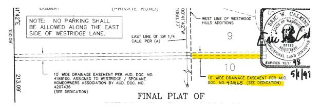
This drainage easement was intended to be the overland emergency discharge for the large tract area where stormwater on this PUD would be captured, treated and discharged; however, as a confined basin, a discharge point was desired. The proposal for our current application is the same with all stormwater being discharged to the large tract in the middle, which also contains wetlands and wetland buffers.
