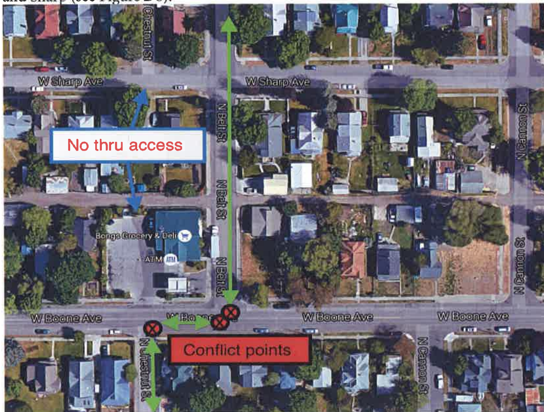
Figure D7 – A diagram showing the three potential vehicle-cyclist conflict points at N Chestnut St, W Boone Ave, and N Belt St.
