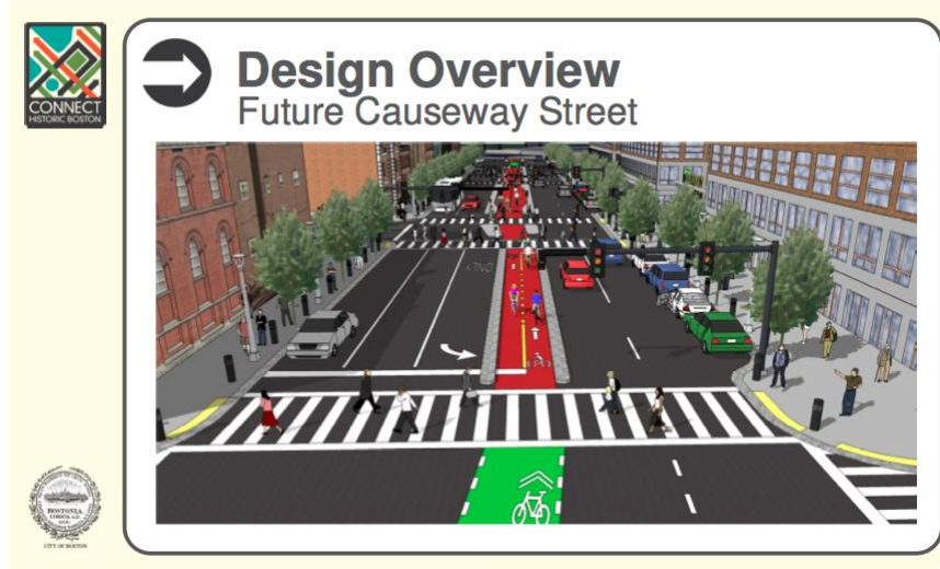
Figure 5.3.4D Image showing potential central, curbed two-way bicycles lanes with painted asphalt. Boston, MA
