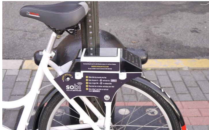
Figure 5.4.4F The Social Bicycle (SoBi) can attach to regular bicycle racks and uses Real Time GPS for tracking. Users can reserve bicycles online.
