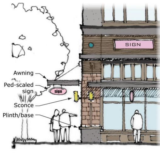
Figure 17C.123.060-A – Illustration of building base, pedestrian scale signs and other building elements described in the FBC.
