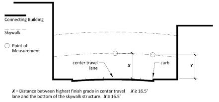
Y = Distance between the top of curb and the bottom of  $Y \ge 15'$  the skywalk structure, at the curb.  $Y \ge 15'$
