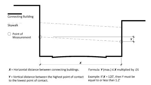
3. No skywalk's structure should have an arch with a rise between the lowest end and the midpoint greater than a five percent slope. (P)
