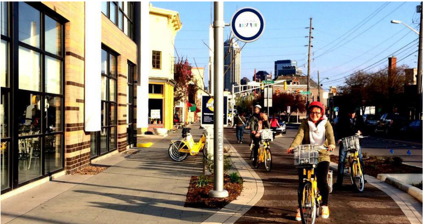
Example of desirable sidewalk environment. Multiple uses can be accommodated on wide sidewalks with distinct paving patterns that denote separate uses.
