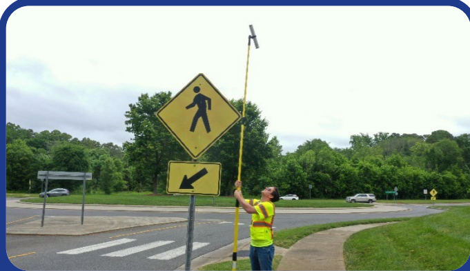
Telescoping poles are used to achieve a minimum 20 feet of camera height.
