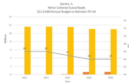
Figure 2-8 - Minor Collector/Local Asphalt Roads $11.618M Annual Budget to Maintain PCI 64
