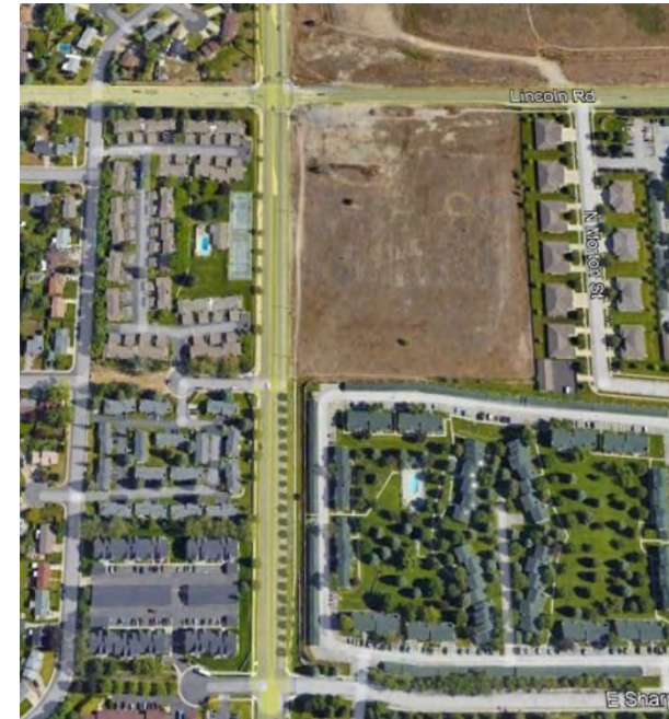
Figure 17. The Lincoln Nevada Neighborhood Center site (vacant property upper center in image) is poorly connected to adjacent residential uses due to the inward facing design of each residential development. The intent of providing stronger connectivity standards is to prevent disconnected development patterns like this, particularly in Centers and Corridors.
