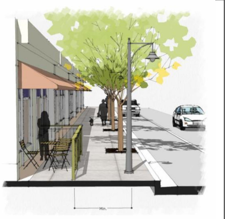
((Figure 17C.123.050-F: Temporary sidewalk encroachments are allowed in the Planting Zone, or in the Clear Pedestrian Zone as per Table 17C.123.050-4.))
