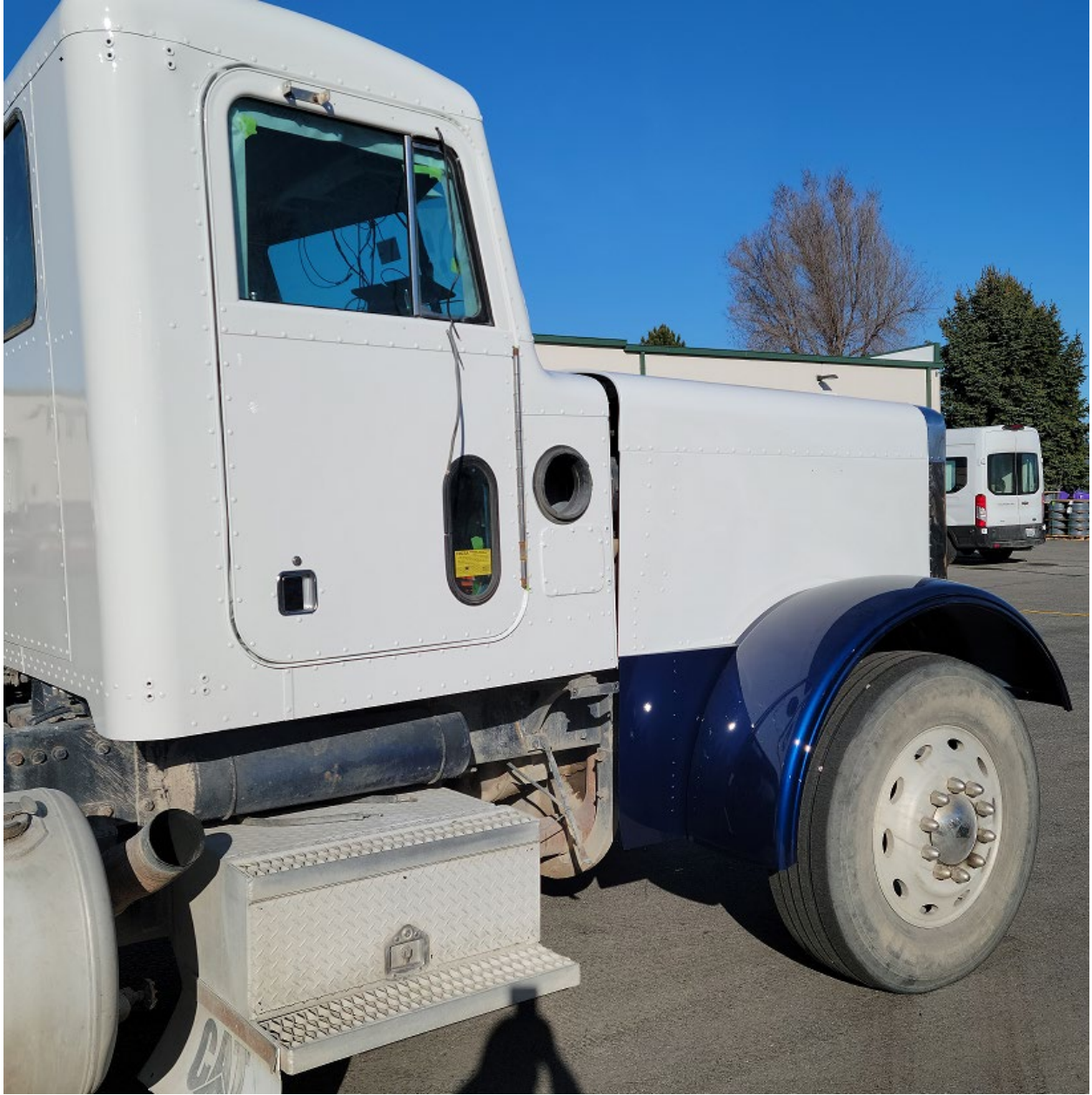
New Hood With New Paint, Cab Re-Spray with body damage repair
