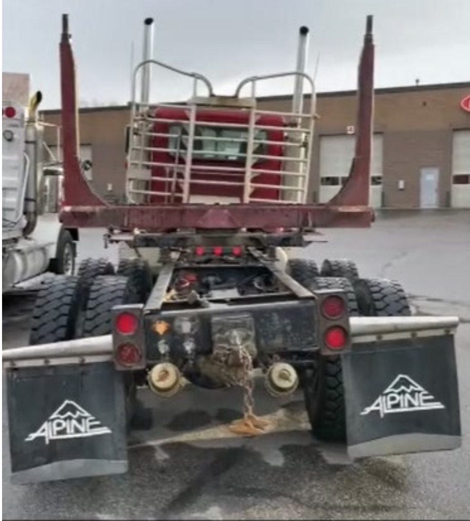
Customer had layed his truck over with a load of logs of the side of the mountain road. We had successfully straighten his frame with a 1/16" bumper to back variance as well as cab to frame.
