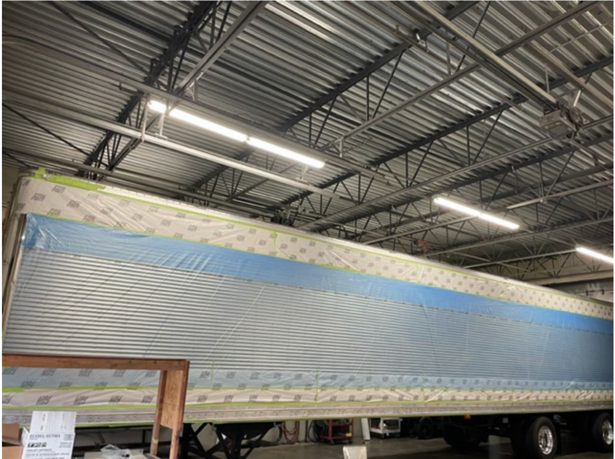
Current Work, Trailer receiving top and bottom rail paint
