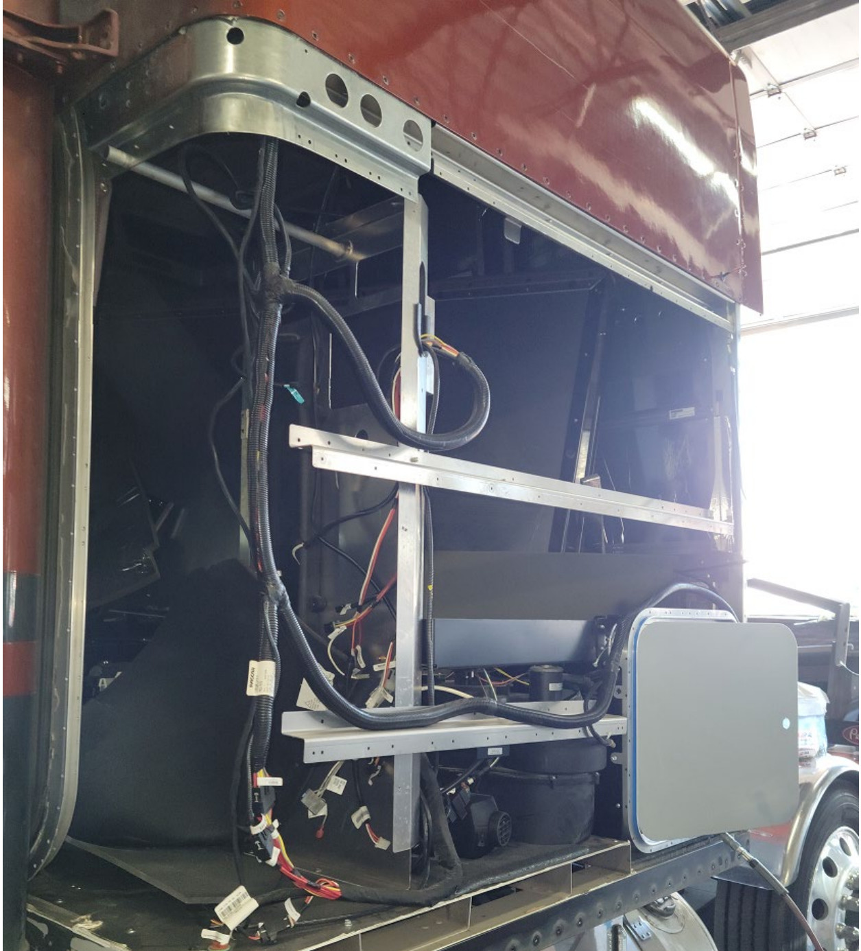
Scratched sleeper side with deformed sheet metal, Re-Skin Replacement and paint.
