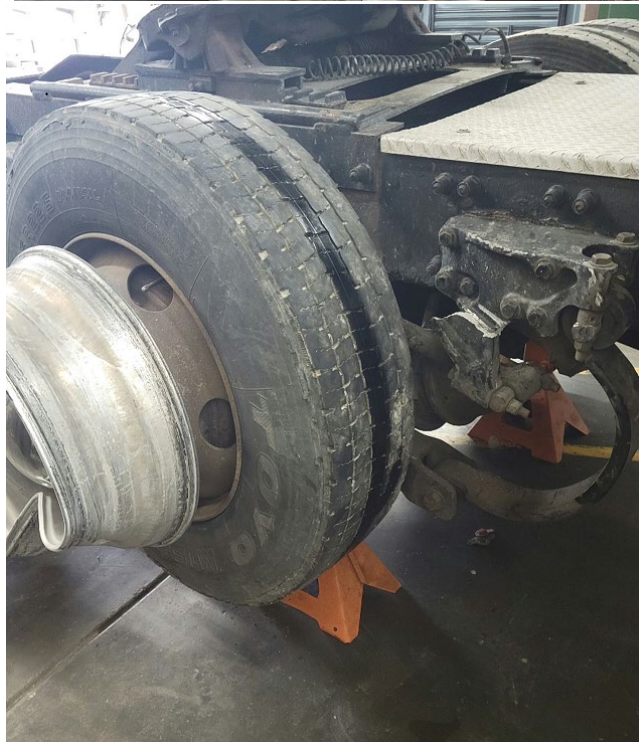
Layover. The Sleeper was able to be repaired without skinning. The truck was loaded and the weight broke suspension parts requiring the front diff housings to be replaced.
