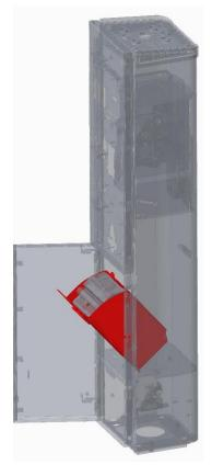
The vault door of the Strada takes up very small sidewalk space and does not go all the way to the ground which is especially important when collecting during snowy conditions.
