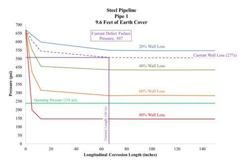
Figure 8 Steel Pipe Performance Curve
