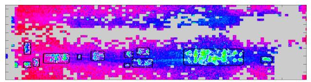
Figure 11. 20-foot Pipe Section – example of coverage – gray indicates missed data
