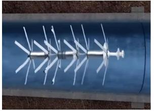
The transducers on the tool create ultrasonic pulses that interact with the pipe wall as the
