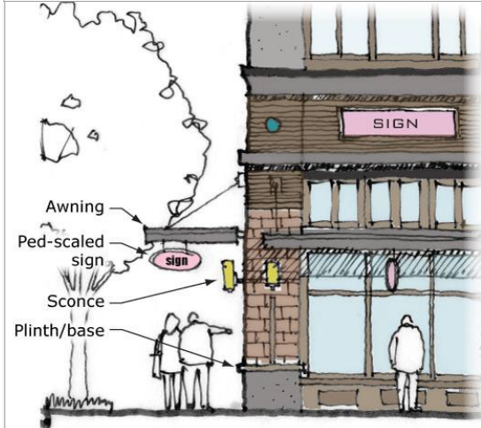
((Figure 17C.123.060-A: Illustration of building base, pedestrian-scale signs and other building elements described in the FBC.))
