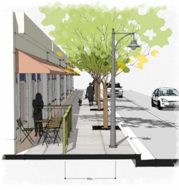
Figure 17C.123.050-D – Temporary sidewalk encroachments are allowed in the Planting Zone, or in the Clear Pedestrian Zone as per Table 17C.123.050-1.
