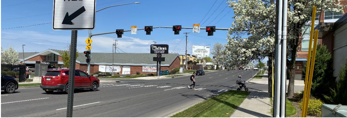
Figure 34. Crosswalk with a HAWK signal on Ruby Ave in Spokane. Source: City of Spokane
