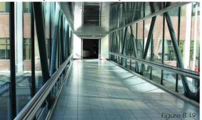
The walking plane on this Spokane skywalk has a slight pitch- but not so steep that a wheelchair could not easily navigate it. Handrails are available to anyone needing a steady hand hold.
