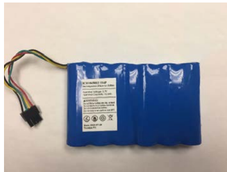
Figure 5 - rechargeable lithium-ion battery pack
