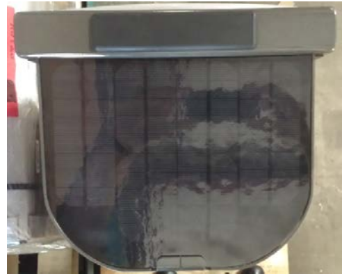
Figure 18 - Integrated solar panel on the top of the MacKay Tango™
