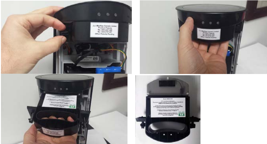
Figure 11 - mkBeacon communications module - easily removed and replaced
