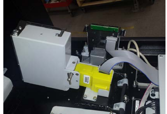
Figure 22 - Easy access to yellow Smartchute™ that can be cleaned or replaced in seconds. Same as coin chute in most MacKay single space meters.
