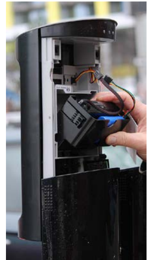
Figure 3 - Maintenance friendly access for on-street servicing
