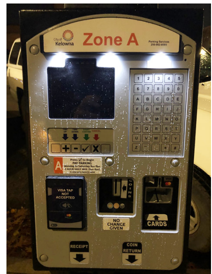
Figure 25 - Faceplate of Tango with optional LED brow light installed for dark hours
