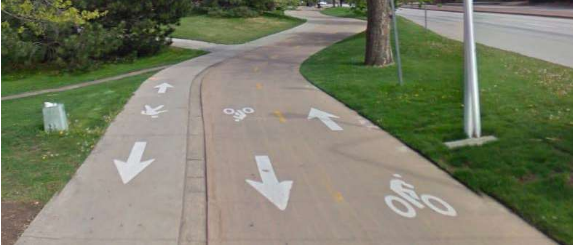
Figure 16 – Shared-Use Pathway with Separate Bicycle and Pedestrian Lanes
