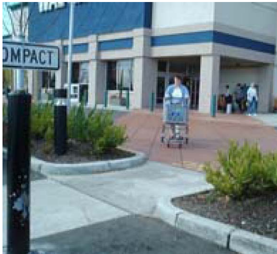
Figure 4.2.2 - Pedestrian Paths may show clear routes to and from building entrances by use of curbs, paving patterns or landscaping.
