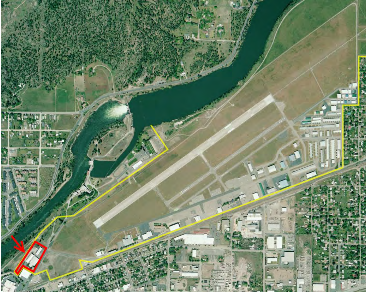
Felts Field Land Purchase in Runway Protection Zone (RPZ) of Runway 4L
