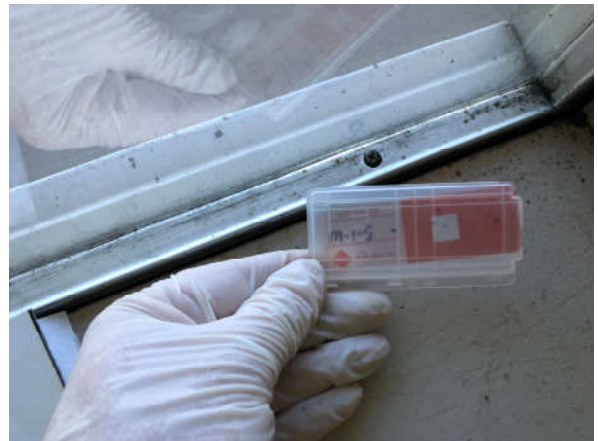
Photo #2 View of mold on window seal in building at 920 Wolverton Court.
